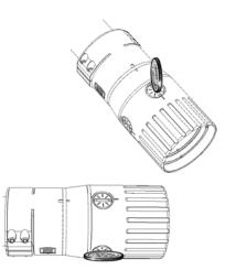
The ScopeX2 utilizes an Adjustment Lock to ensure no loss of zero under recoil. Before adjusting the turrets, remember to loosen this screw with the included 1/16" hex wrench, and to secure this screw when final zero is achieved. Snug this screw lightly with about 5 in/lb of pressure. Do not overtighten.
